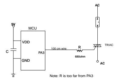
The correct connection should be firstly connecting PA3 to the 680ohm resistor as close as possible, and than the long wire for higher noise immunity.
